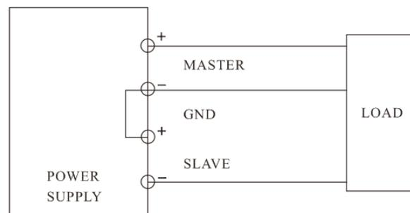
Fig.5-4 Positive and Negative Supply
